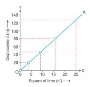
The value of acceleration due to gravity (g) can be obtained by doubling the slope of the  $S-t^2$  graph for a freely falling body.
